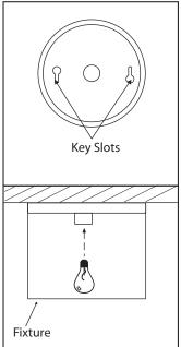
3. Once wire connections are completed, carefully tuck wires and wire nuts into the outlet box making sure no bare wire (on the black and white) is visible at the wire nuts. Tuck the electrical wires into the electrical box and position the "key slots" over the support screws. Turn and lock the support screws into the "key slots". Tighten the support screws into place.
