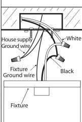
2. Firmly attach the fixture ground wire (bare copper) to the mounting bracket with the ground screw (by wrapping around the ground screw) and then connect it to the house supply ground wire with a wire nut. Connect the black wire (or wire with marking) from the fixture to the black wire in the electrical box and connect the white wire from the fixture to the white wire in the electrical box.
