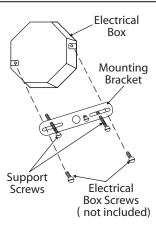
¶ o Install the mounting bracket to the electrical box using two electrical box screws. (Note: Do not adjust the two support screws at this time.)
